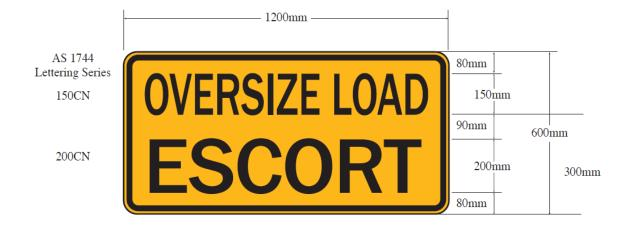
Figure 5 - Escort Vehicle Warning Sign on Vehicle
